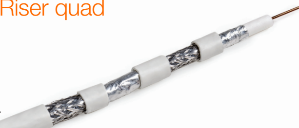
Câble coaxial, RG6, quad, 18 AWG, 3.0 GHz, 60% tressé, coté CMR
