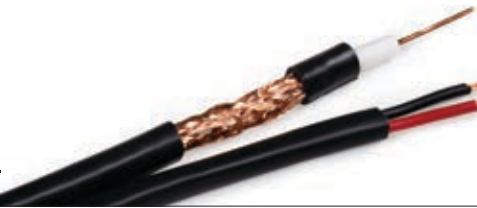
Coaxial Cable, RG59/CU, Siamese, 95% Braided, 18/2 AWG, CMR Rated Available in: Part no. COAX-RG59/CU-Siamese-CMR-XX-305 (1000 FT Reel)
